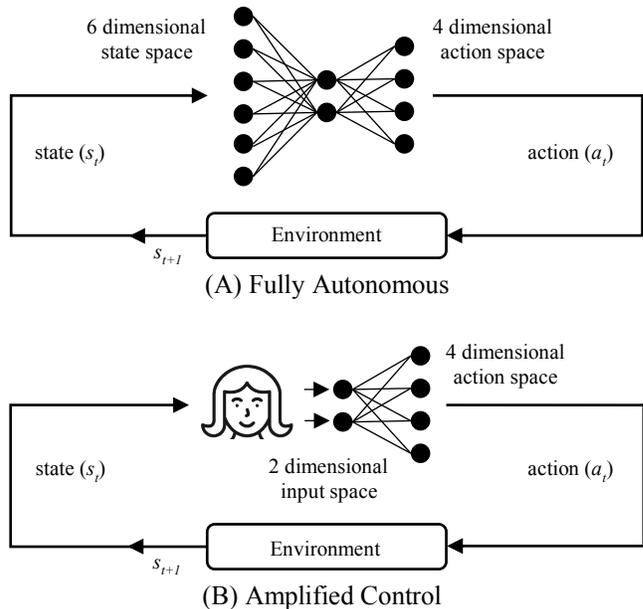
Fig. 1. Our approach to amplified control uses deep neural networks and consists of two steps: (A) training a deep neural network, and (B) replacing the front half of the network with a human user.
