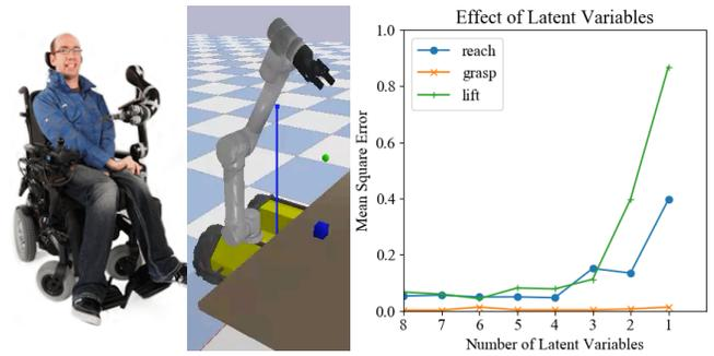
Fig. 2. JACO robotic arm mounted on a power wheelchair [3] (left), our simulation environment (center), and preliminary results (right)
