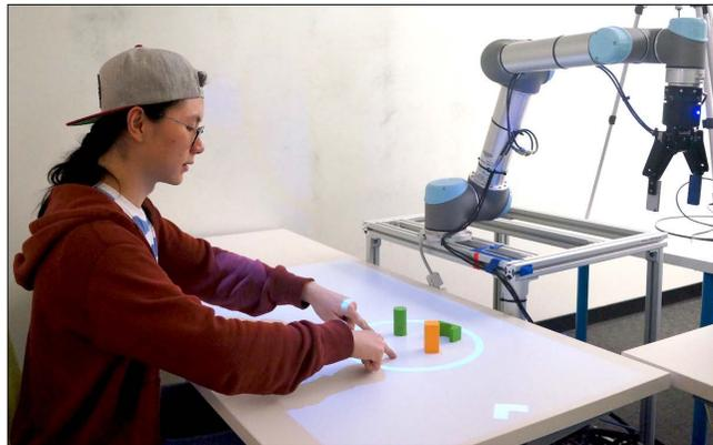
Fig. 1. PATI supports the augmented and situated specification of robot tasks, allowing users to teach their robots new tasks by directly referencing and interacting with the environment through tools (e.g., shape tools) and common touch screen gestures, such as pinch, tap, or drag-and-drop.
